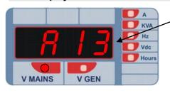
In case of alarm, the display shows a alarm identification code: the alarm led turns on.
